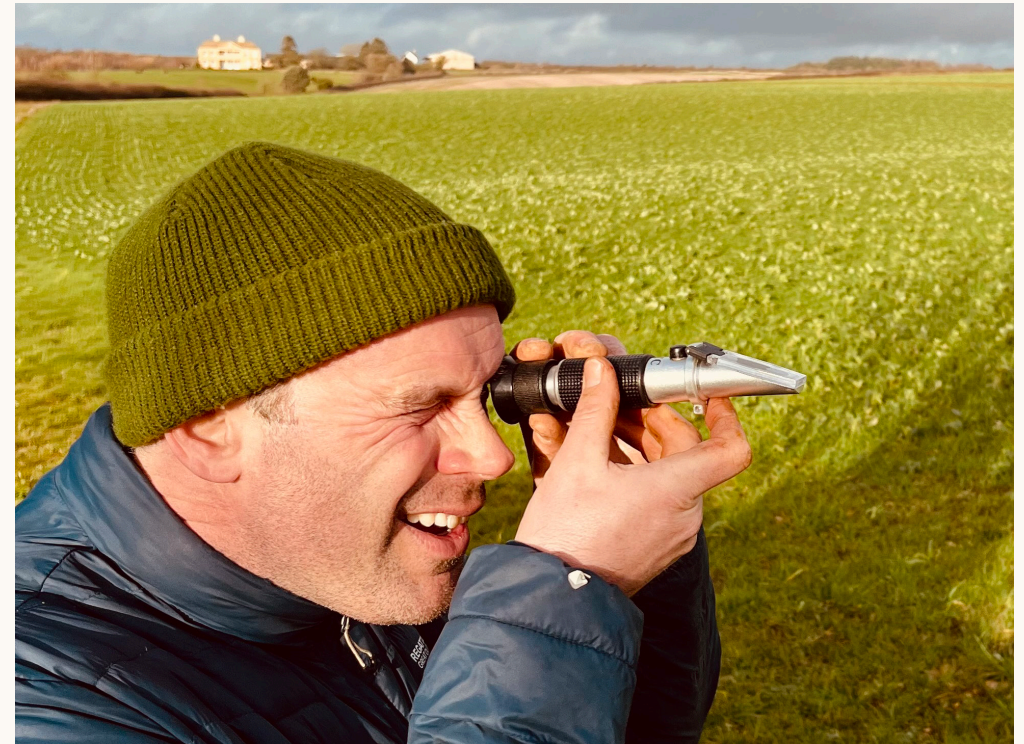
SAM PHILLIPS TESTING HIS BRUX WITH HIS PORTABLE REFRACTOMETER
